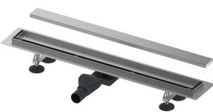
**TECElinus shower channel set, extra flat, "2 in 1" cover, with membrane odour trap****Article number:** 15106089**Nominal length:** 800 mm**Total length L:** 800 mm**Visible dim. after installation:** 740 mm**Width in unfinished state:** 135 mm**Visible width****after installation:** 75 mm**DU 1:** 1 pc.**DU 2:** 40 pc.**Description:**
