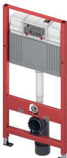
**TECEbase toilet module with Base cistern, including TECEambia bright chrome toilet flush plate, installation height 1120 mm****Article number:** 9400405**DU 1:** 1 pc.**DU 2:** 10 pc.**DU 3:** 60 pc.**Description:**
