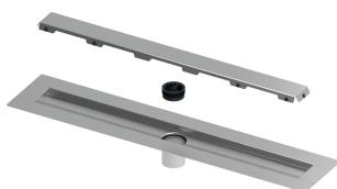
**TECEshowerline shower channel for natural stone, straight, with stainless steel support as a set****Article number:** 15201072**Nominal length:** 700 mm**Total length L:** 735 mm**Support sheet****length L - 89:** 646 mm**Covering cut-out****length L - 87:** 648 mm**Visible width****after installation:** 626 mm**Width in unfinished state:** 152 mm**DU 1:** 1 pc.**Description:**
