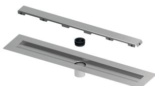
**TECEshowerline shower channel for natural stone, straight, with stainless steel support as a set****Article number:** 15201082**Nominal length:** 800 mm**Total length L:** 835 mm**Support sheet****length L - 89:** 746 mm**Covering cut-out****length L - 87:** 748 mm**Visible width****after installation:** 726 mm**Width in unfinished state:** 152 mm**DU 1:** 1 pc.**Description:**
